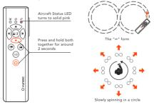
TIPS: Keep distance from magnetic interference during the calibration. We recommend calibrating Wizard outdoors. You can find the TYPHOON Wizard calibration tutorial video at www.yuneec.com/wiz-info.html
